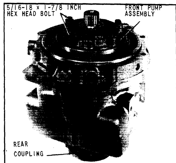
Fig. 100 Bolting Front Pump Assembly
